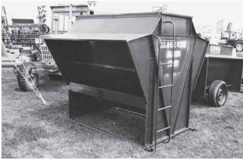
A grain self-feeder for cattle allows continuous access, but slow supply, of free flowing feeds. The feeder trough is protected from the rain.
