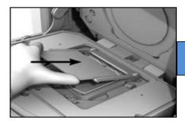
Load PicoTiterPlate device on instrument
